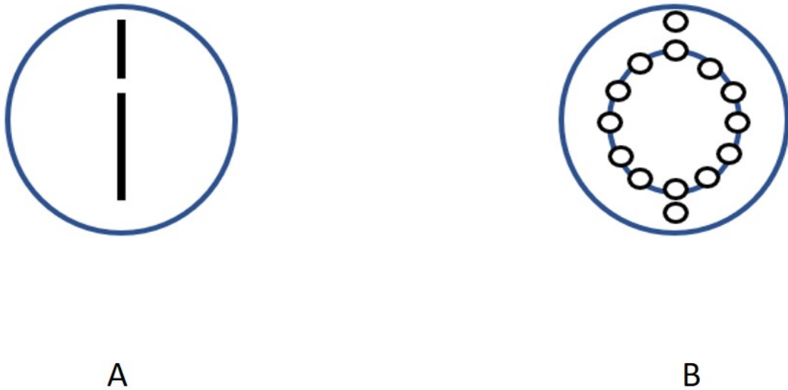
FIGURE 2.3: Schematic diagram of hybrid selection valve. The rotor (A) and stator (B) are shown.
